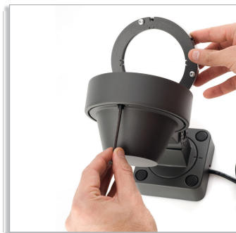
Opening the rear cover of a DCP623/624
